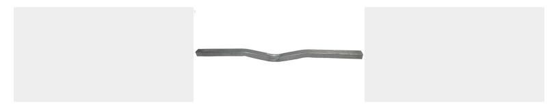
Heavy-duty hot-dipped galvanized drop center cross member with 7 gauge nominal wall thickness. Measures 3" wide x 3" high. It has no pre-drilled holes.
